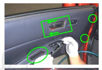
To gain access to the door catch you will have to remove the speaker.
