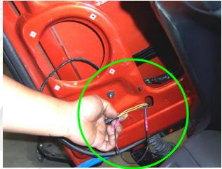
You will have to extend the wires going to the mirrors. Use the included wires.
