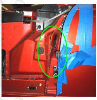
Use a hammer the bend the left side first and then the right side so that they form a flat surface and layer one on top of the other.
