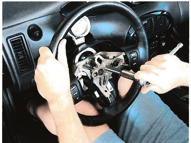
Fig. 6 - Use the steering wheel puller to draw the steering wheel off the steering column shaft..
